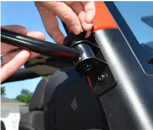
Figure 4: Install mirror arm and bushing with knob and washer.
