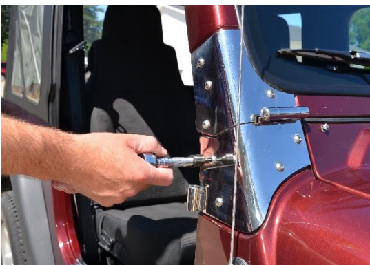
Figure 2: TJ - remove lower T40 Torx bolts.
