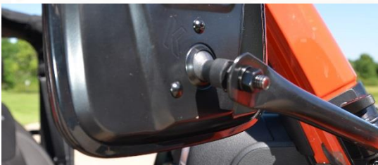
Figure 5: Mirror head installed on mirror arm assembly.
