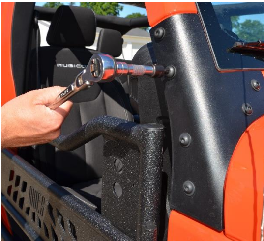
Figure 1: JK - remove upper two T40 Torx bolts.
