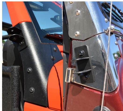
Figure 3: Ensure weldnut is facing down.
